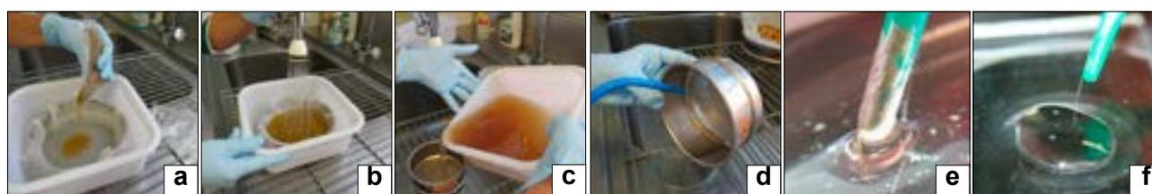
Figure 1. a–f Nematode extraction by filtration method.
