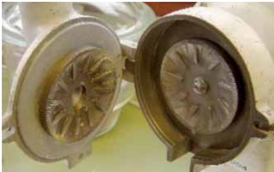
Figure 3: The Regent-Maskin grinder has two fixed grinding plates one of which rotates when the electric motor is switched on.
