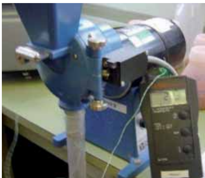
Figure 9c: When grinding starts with the Janke & Kunkel the temperature of the ground material is just above ambient.
