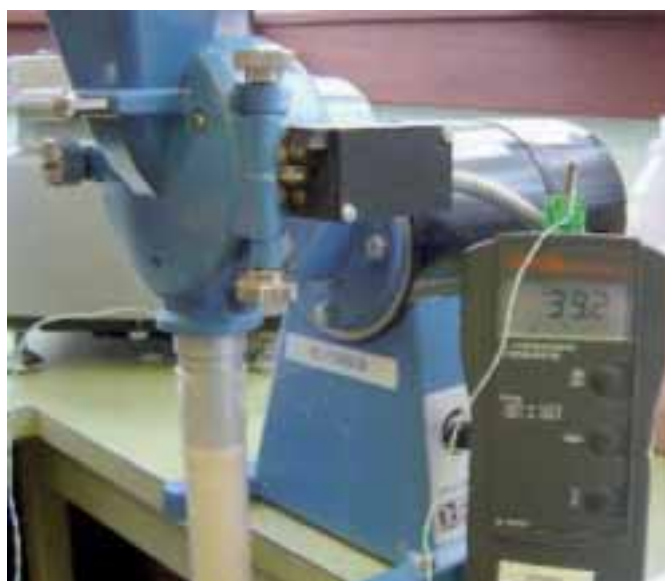
Figure 9d: After grinding one oat replicate, the temperature of the second replicate to be ground is nearly 40°C.
