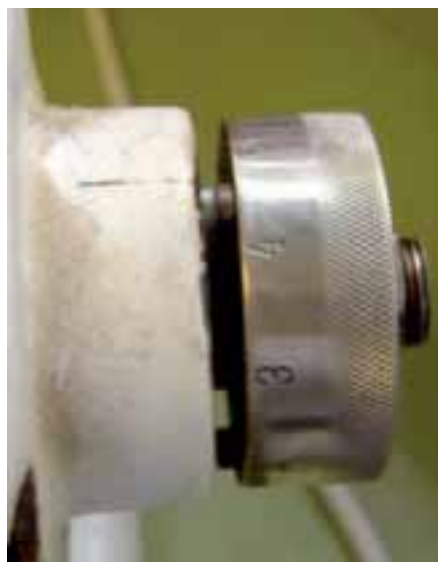
Figure 4: The distance between the plates can be adjusted to give fine or course grinding. Unfortunately even with the grinder set at No 1 with the plates touching it does not grind to the fineness required in the ISTA Rules.
