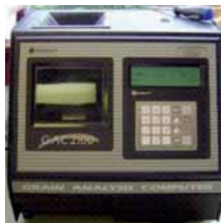
Figure 1: The Dickey John GAC 2100 Grain Analysis Computer used to measure the moisture content of the cereal seed samples used in this grinder performance trial.
