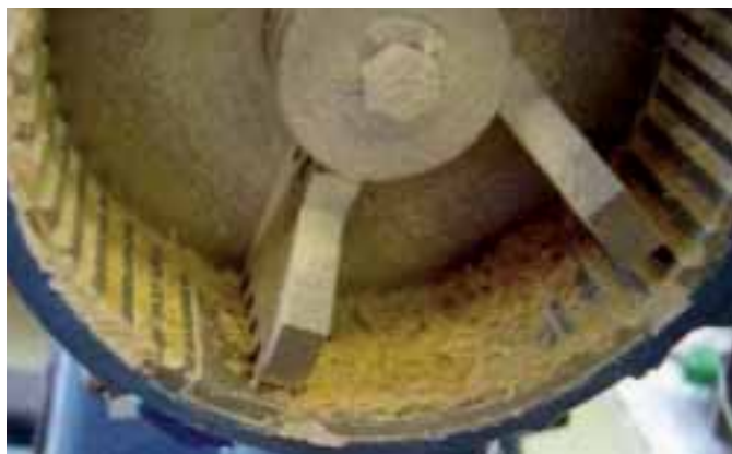
Figure 9a: Husks and coarse particles are retained in the drum of the Janke & Kunkel hammer mill.
