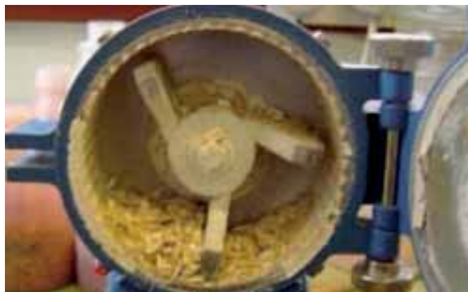
Figure 9b: The Janke & Kunkel grinder can become blocked with husks obstructing holes in the internal sieve.
