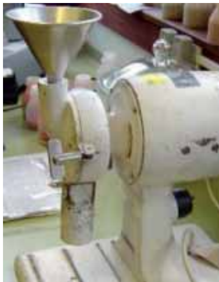
Figure 2: The Regent-Maskin grinder.
