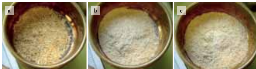
Figure 6: Material from ground oat sample retained on 1.00 mm sieve (a), 0.5 mm sieve (b) and that passing through 0.5 mm sieve (c).
