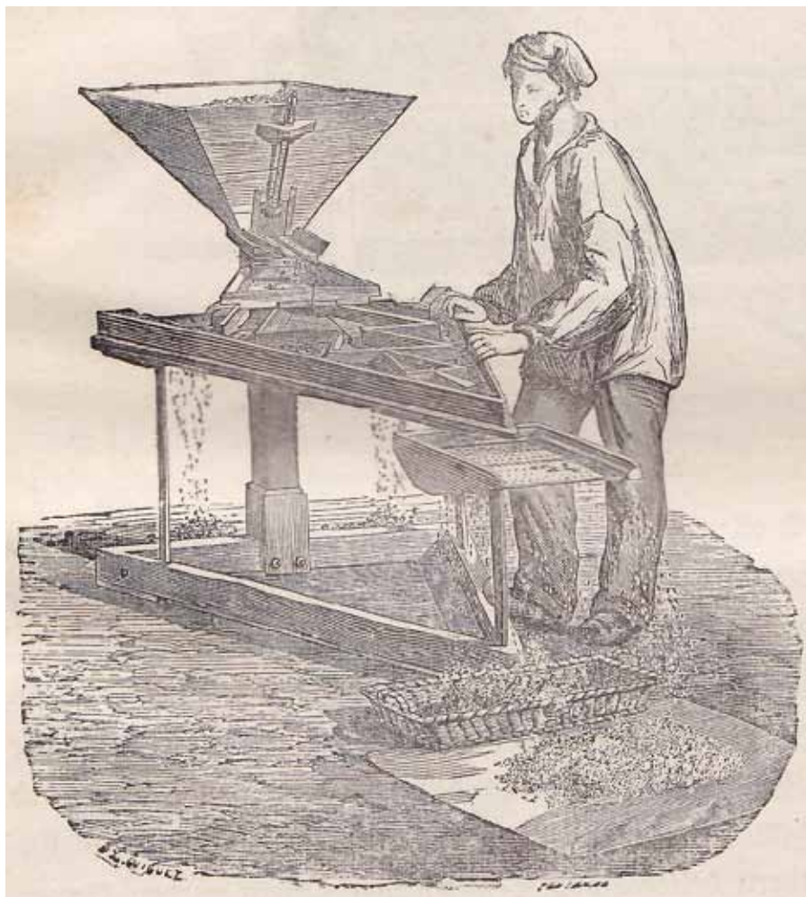
Figure 3. The gravity separator of Josse, Ormesson-sur-Marne (now Val-de-Marne, France) as exhibited by Hignette (Paris, France); from Nobbe, 1876.
