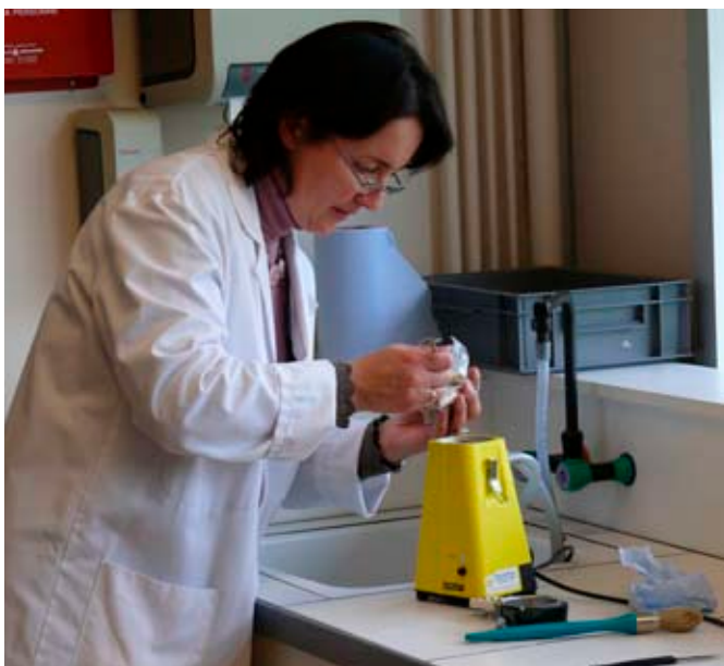
Grinding in preparation for moisture testing
