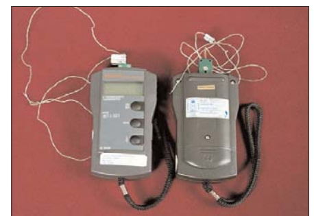
Plate I Calibrated electronic digital thermometer used to check oven temperature and oven temperature profile when conducting Moisture Content tests
