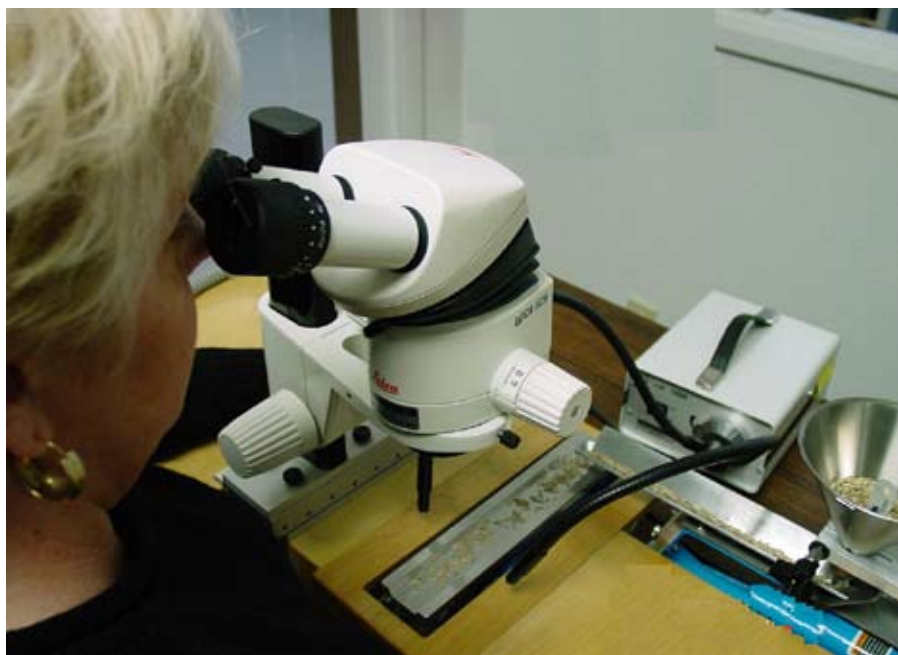
Figure 4. The Ergo Vision System being used. The analyst sits in an ergonomically correct position and uses both eyes at optimum magnification, the seeds flow continuously and the process can be started and stopped any time to remove contaminants.
