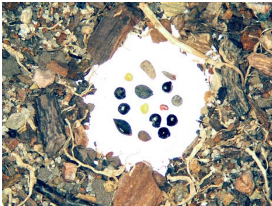
Figure 5. A new application of the Ergo Vision System is the determination of seeds in the soil-seed bank tests at OSU Seed Laboratory. Due to the preliminary preparation of the sample, notice that seeds are clearly distinguishable and the rest of the sample does not look like soil any more.
