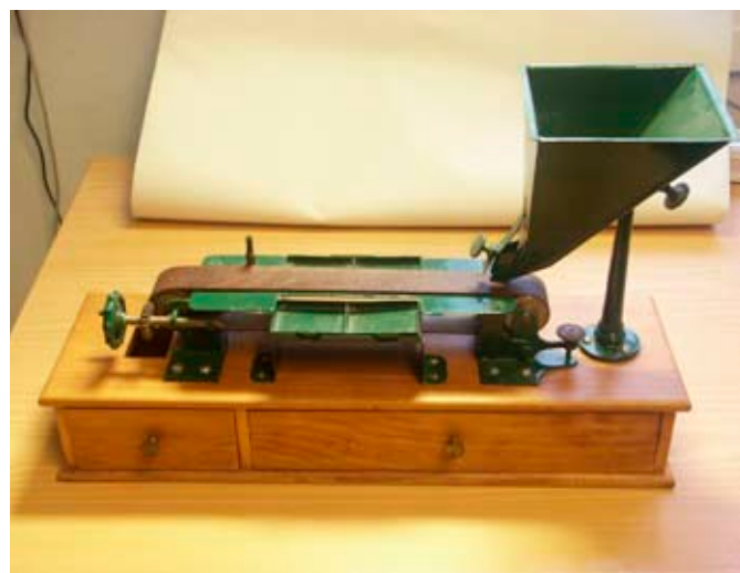
Attempts have been made to mechanize the purity analysis, e.g. with devices which transport the seed sample under the magnification glass, by use of vibrators moving the seeds to be inspected under a microscope (Oregon Inspection Stations), or under a seed scanner with built-in sorting of the seeds. Above: two old models from Sweden (photos supplied by Karin Johansson).
