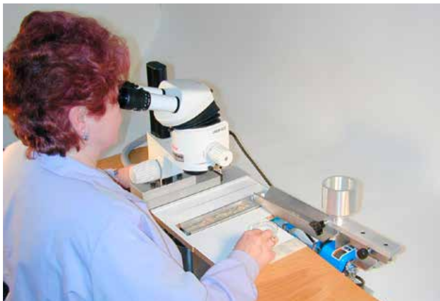
Figure 2. Purity testing using the Ergovision system, with features including an ergonomic position for analysts, high quality optics, lights, and a mechanical seed feeder.
