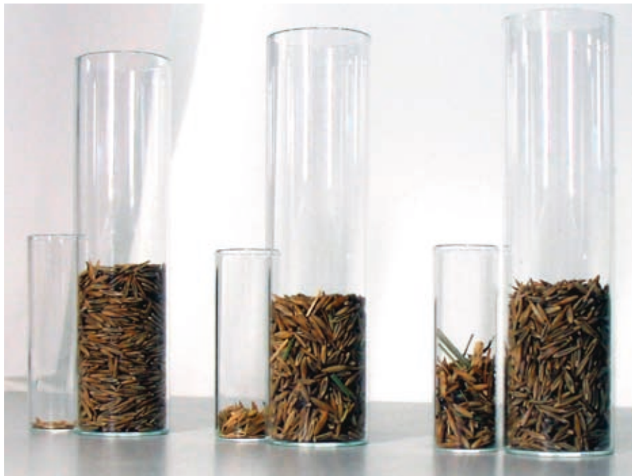
Figure 10. Three samples of tall fescue blown at the same EAV value. Small vials contain the light fraction (blowings), and large vials contain the heavy fraction (pure seed). Separation occurs regardless of the amount of the light materials present in each sample.
