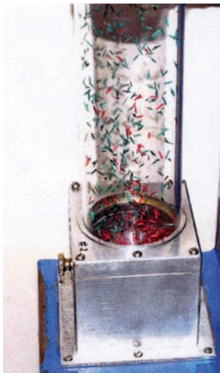
Figure 7. Master calibration samples are used to find the correct air-gate opening to provide the optimum blowing point to achieve separation of empty (green) and pure (red) florets.
