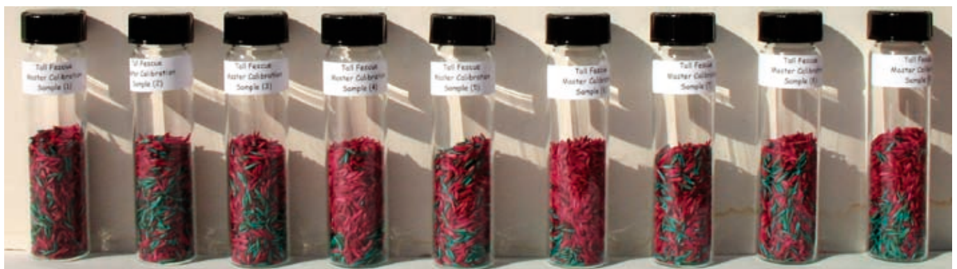
Figure 6. A set of tall fescue master calibration samples where green florets represent empty seeds and red represent pure seeds. Every individual sample in the set has the capacity to find the same optimum blowing point.
