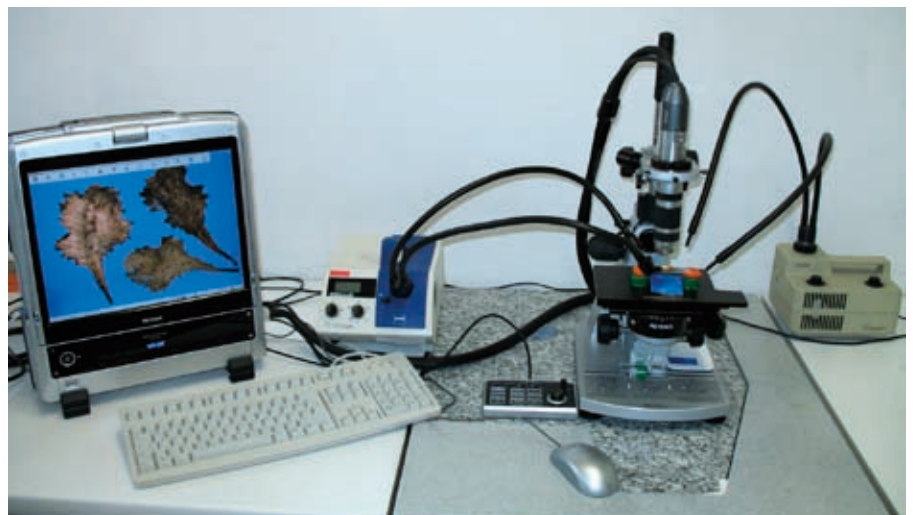
Figure 1. The Keyence microscope (all photographs ©LTZ Augustenberg, Karlsruhe)
