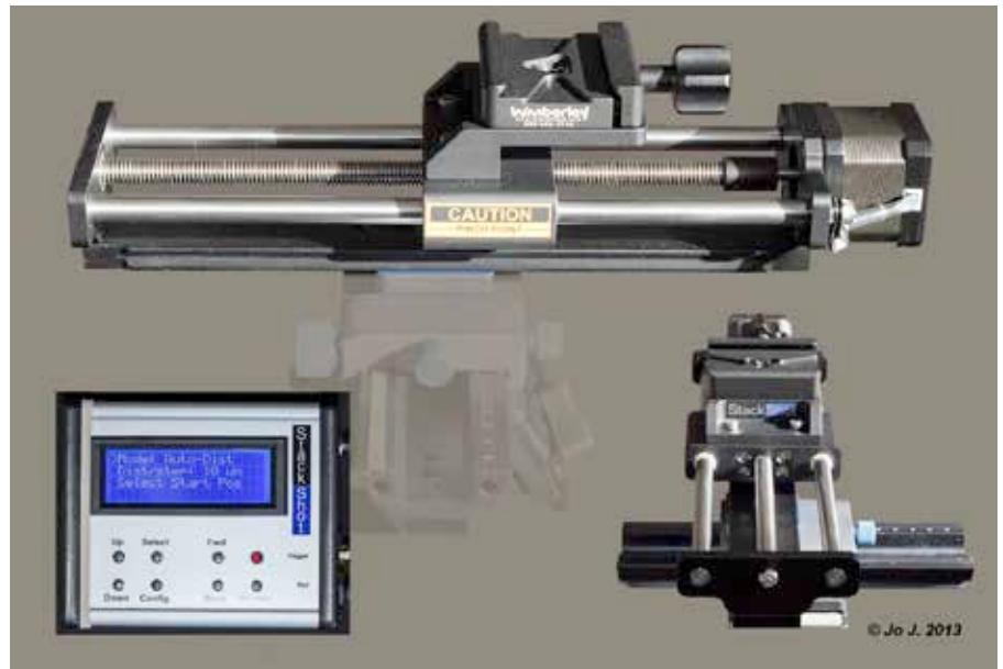
Figure 4. My arrangement for the StackShot and Controller. I also use a Novoflex macrofocusing rail to facilitate movement along an axis at 90° to the StackShot. For easy attachment of the StackShot to the Novoflex rail and the camera to the StackShot I use quick release platforms and plates from Novoflex and Wimberley. The Novoflex rail is attached to a tripod using a ballhead, again with a quick release plate.
