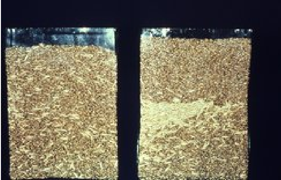
Bag prior to Vibration Bag after vibration applied to top of bag
