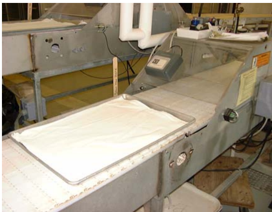
Figure 1. Germination tray covered with crepe cellulose paper (Versa-Pak®) moving through a water sprayer table.
