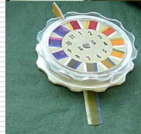
Using pH paper to measure the pH of paper germination media.
