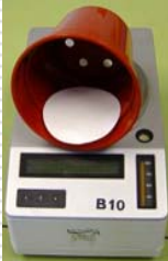
The germination media is weighed. For sand and organic growing media a waterproof container with drainage is required. The drainage holes are covered using a material that allows water drainage but prevents the loss of material
