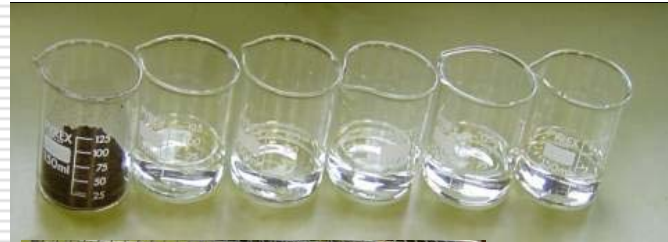
For Paper Media samples are moistened, with water that is to be used for germination tests 1 and the pH is measured on the surface of the paper.
