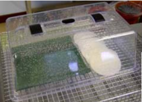
The Germination media is saturated with water and allowed to freely drain for 12 hours with measures being taken to prevent evaporation. The saturated media is then weighed and the maximum amount of water held in the growing media as percentage of its dry weight is calculated
