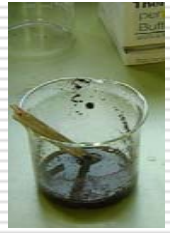
For Paper Media samples are moistened, with water that is to be used for germination tests 1 and the pH is measured on the surface of the paper.
