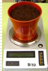
The germination media is weighed. For sand and organic growing media a waterproof container with drainage is required. The drainage holes are covered using a material that allows water drainage but prevents the loss of material
