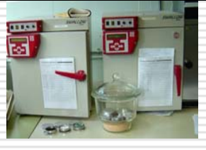
The Moisture Content of the Germination media is measured using the ISTA Constant Temperature Oven method at 130°C
