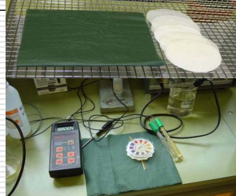
For Paper Media samples are moistened, with water that is to be used for germination tests 1 and the pH is measured on the surface of the paper.
